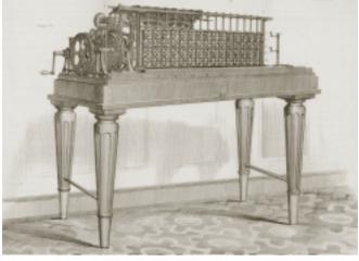
The observatory was outfitted with the finest equipment of the time, including this Scheutz difference engine, a pioneering effort to automate scientific computation.
